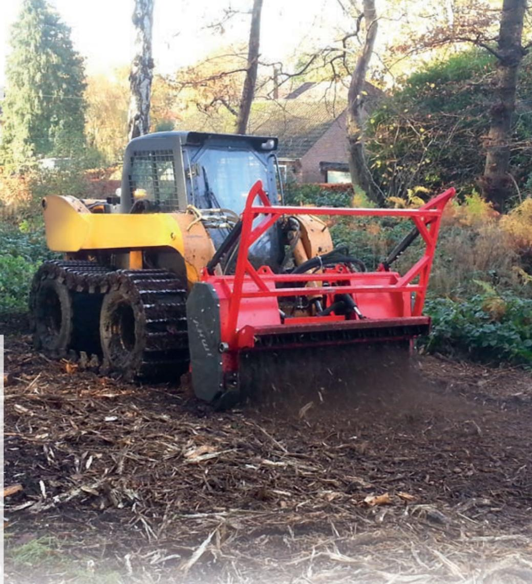
The M450h is a lightweight mulcher for universal use with skid steer loaders in the power range of 80–130 hp.
